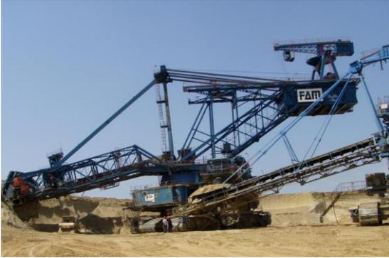
**Fig. 1.** SRs2000 Bucket Wheel Excavator
